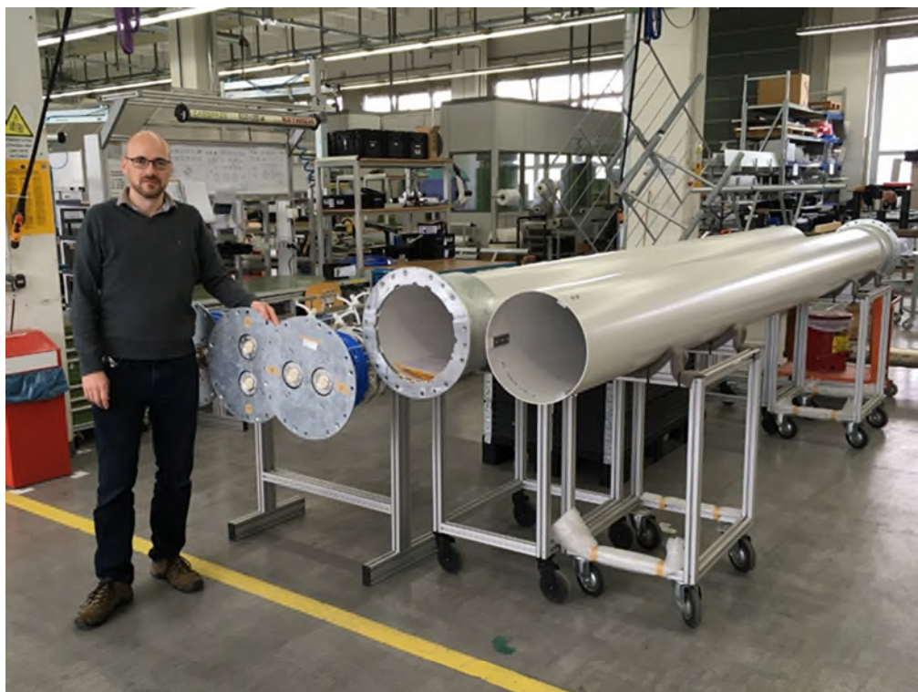
in the picture: Markus Gerl, project manager for the US market in front of a series of new dual polarized omni antennas. Notice: the two separate inputs for H- and V-pol.
